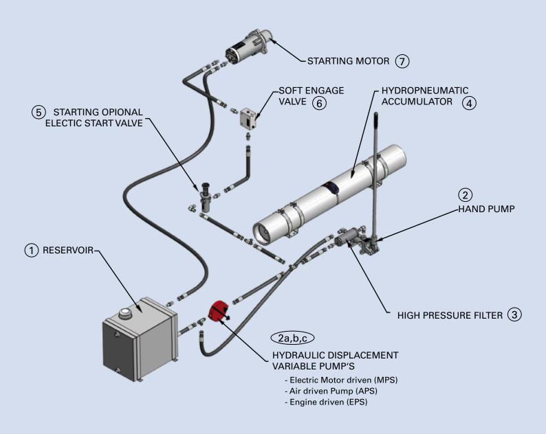
From a reservoir (1), or from an existing hydraulic system, hydraulic fluid is pumped, either manually (2), or by some auxiliary pump (2a,b,c), into a virtually maintenance-free accumulator (4). In it is a free floating piston, which is under nitrogen gas pressure, pre-loaded to c.100 bar.
